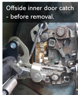
Offside inner door catch (removed).
