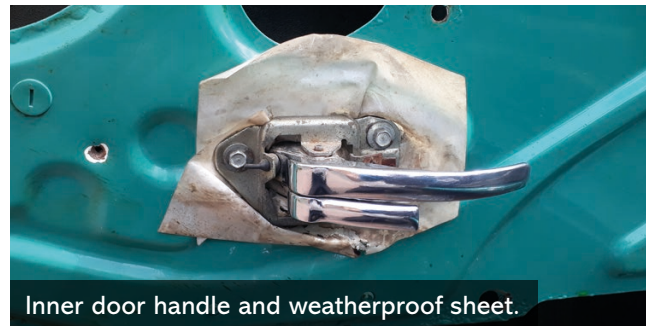
Offside inner door catch (removed).
