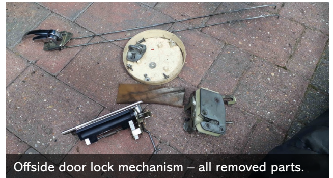
Outer door handle inner mechanism.
