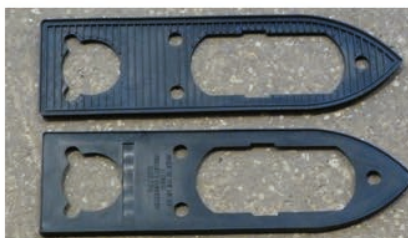
Rear Lamp Gasket Part No 216126
