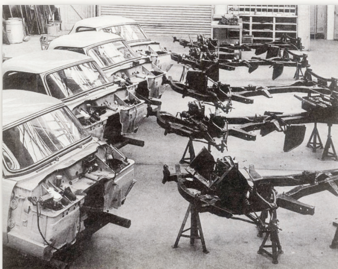
Four competition Spitfires being built in the workshop. These are the bodies of the rally cars with the 'bubble' hard tops ready to be dropped onto the chassis.
