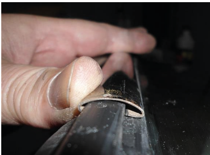
Fig. 3 – This shows a mismatch between the protrusion on the rubber surround and a trim strip which has only about 4mm turned over on each edge. The tendency is for it not to be securely held behind the protrusion and it will not fit firmly. (pic from the Forum)
