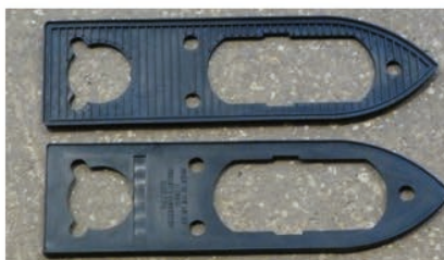
Rear Lamp Gasket Part No 216126
